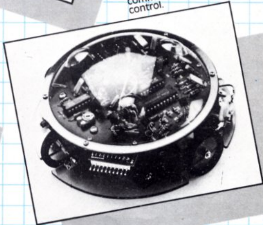
Circular £29.99 Through its own hand-held remote control you issue instructions to the two independently driven wheels - sending the circular wherever you want it to go.
